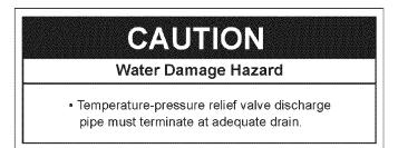
No valve or other obstruction is to be placed between the relief valve and the tank. Do not connect tubing directly to discharge drain unless a 6 inch air gap is provided. To prevent bodily injury, hazard to life, or property damage, the relief valve must be allowed to discharge water in quantities should circumstances demand. If the discharge pipe is not connected to a drain or other suitable means, the water flow may cause property damage.
